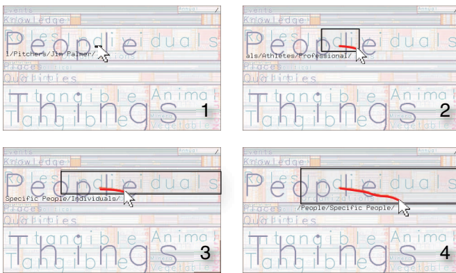
Figure 5. Direct access navigation. A crossing-based interaction enables direct access to visible nodes.
